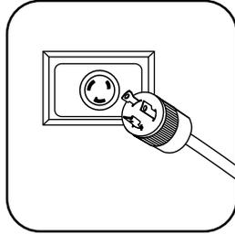
AC Input Connection: Insert L6-20P locking plug into compatible L6-20R utility, generator or UPS outlet. For international applications, connect user-supplied power cord with region-specific plug to C20 power inlet.
