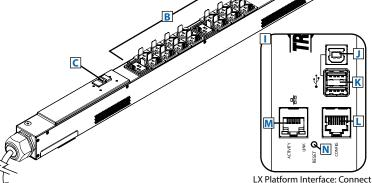
to 10/100/1000 Mbps Ethernet networks for remote monitoring via SNMP, Web, SSH, or Telnet. \*Add optional EnviroSense2 (E2) modules for temperature, humidity, and dry contact signaling.
