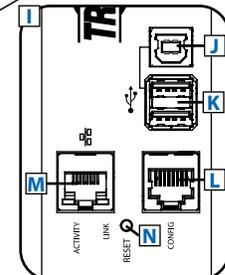
LX Platform Interface: Connect to 10/100/1000 Mbps Ethernet networks for remote monitoring via SNMP, Web, SSH, or Telnet. \*Add optional EnviroSense2 (E2) modules for temperature, humidity, and dry contact signaling.
