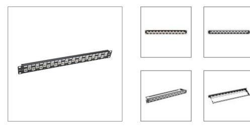
24-port Cat6a patch panel with staggered RJ45 ports manages and organizes Cat6a input and output cable connections and reduces crosstalk in your high-density 10 Gbps Ethernet network. 110 punchdown termination required.
