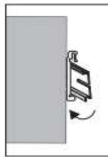
Removing the Switch
