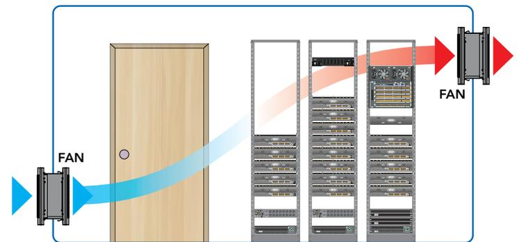
(2) SRCLOSETFAN fans installed on opposite sides of the room, one for inflow and the other reversed for outflow.
