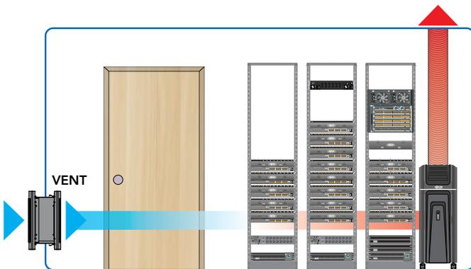
SRCLOSETINTAKE for inflow combined with a portable cooling unit like the SRCOOL12K that vents warm air via its duct.
