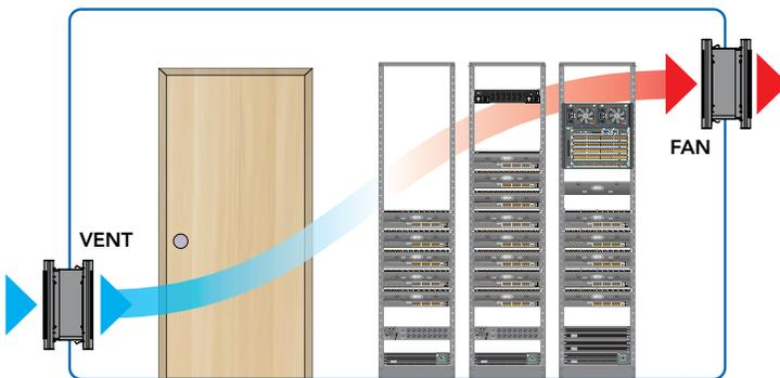
SRCLOSETFAN fan installed high on the wall to expel warm air combined with a SRCLOSETINTAKE vent installed on the opposite side of the room to allow cool air to enter from outside.
