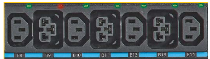
Green LED indicates power on and red indicates power off to outlet.
