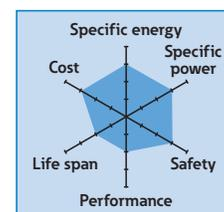
Lithium Manganese Oxide (LiMn<sub>2</sub>O<sub>4</sub>) - LMO
