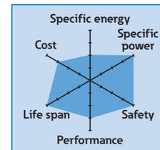
Lithium Iron Phosphate (LiFePO<sub>4</sub>) - LFP
