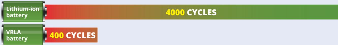
\*Discharge cycles for lithium-ion battery and VRLA batteries in Eaton 9PX UPS systems @ 25°C (77°F)
