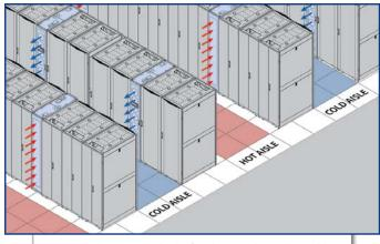
Drawing in hot air at the back of each row and providing cold air at the front of each row, **SRCOOL60KCW** is a perfect match for efficient hot-aisle/cold-aisle data center configurations.
